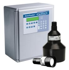
**DESCRIPTION** The SonoTracker<sup>TM</sup> Ultrasonic Level System can monitor up to 16 vessels with transducers of various frequencies, and vessels of different heights and shapes and accurately measure the level of many different materials. It allows you to read levels from 1 foot to beyond 100 feet in solids, and additionally the same unit can be used for open channel flow and differential level measurements.
