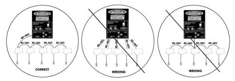
The recommended communication cable is Belden #9842 (2-pair, AWG 24) or equivalent. Using this
